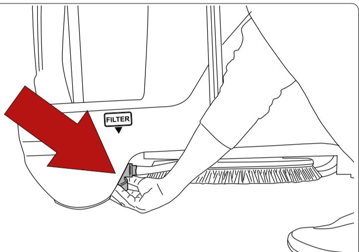
Check that the detergent outlet filter is clean.
